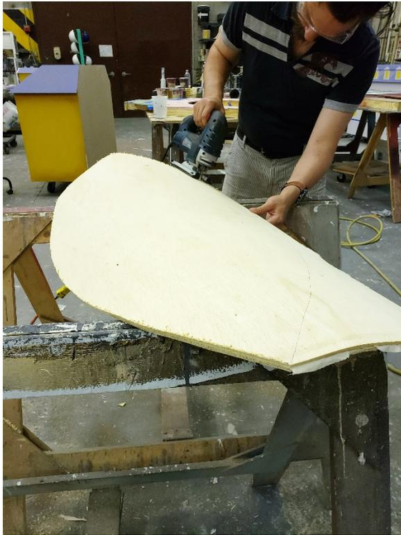
Use a jigsaw to cut out the shape of the traced pattern (remember your eye protection!).
