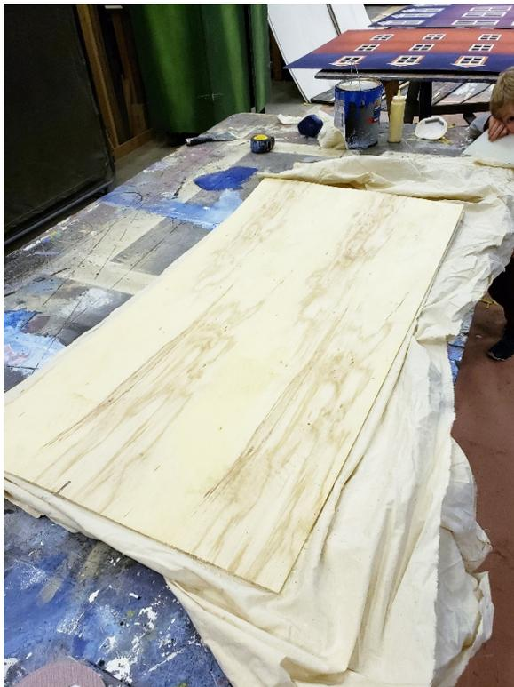
Take the second sheet of plywood and lay it on top of the muslin. We've now made a sandwich of two sheets of plywood with muslin in between. Two sheets of plywood will give us the mass we need and will allow us to bend the boards into place. The muslin
