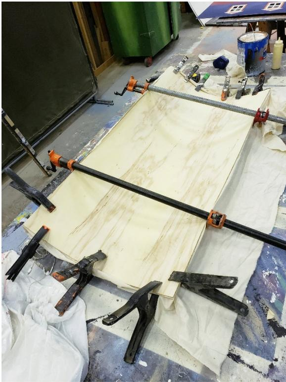
between prevents the boards from cracking. Clamp the perimeter of the plywood while the glue dries. We used two long clamps across the width to bend the plywood into place. Straps can also be used to get the desired curvature.
