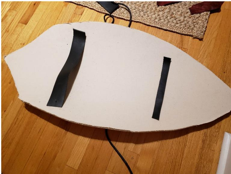
Cut the canvas to the edge of the shield using a box cutter. Place the leather straps on the back side and mark their placement. The top strap should be just below the armpit while the small strap should be an arm's length away so the hand can grasp it.
