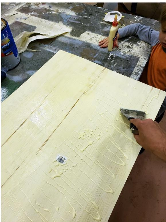
Start by coating one side of the plywood sheets with wood glue. Here we're using a trowel to spread the glue evenly over the entire sheet.
