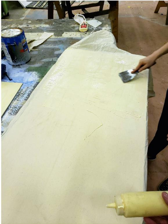
Coat the top side of the muslin (which is now glued to the first sheet of plywood) with wood glue in the same manner as we coated the plywood.
