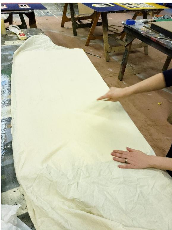
Take your muslin and spread it over the plywood, making sure the entire sheet is covered. We used a flat edge of a thick piece of plastic to push the muslin into the glue and eliminate any wrinkles.
