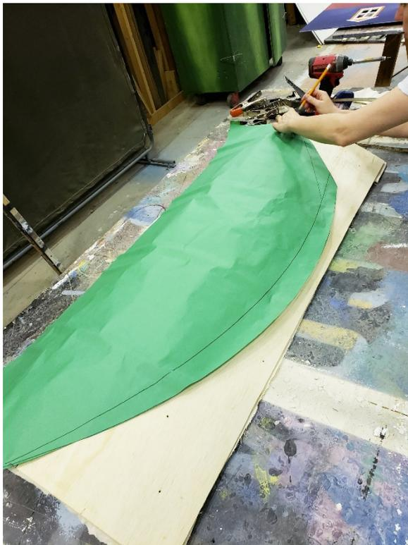
Mark the center of the plywood on both the top and the bottom. Trace half the shape of the shield on paper or any extra muslin. Place that 'half' pattern on one half of the plywood and trace it onto the wood. Flip the pattern and repeat on the other half.
