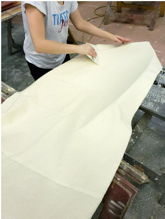
Lay the canvas over the glued side. We used the same flat edge of a flat piece of plastic to press the canvas into the shield and to remove and wrinkles.
